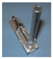
Figure 47 Electrospray nebulizer needle in needle holder
