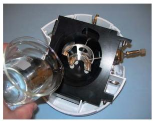
Figure 7 Filling the spray chamber
