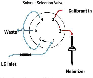
Figure 3 Calibrant to LC/MS flow
