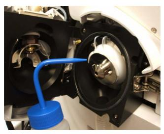
Figure 24 Rinsing the area around the spray shield
