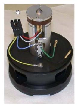
Figure 69 The re-assembled ion optics assembly
