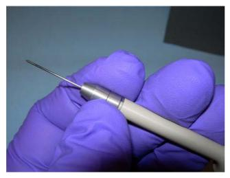
Figure 45 Unscrew the corona needle from the shaft.
