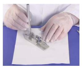
**Figure 15** Nebulizer installment with the adjustment fixture.
