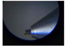
Figure 37 Corroded needle in nebulizer
