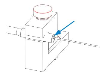
Figure 52 New capillary in the capillary guide
