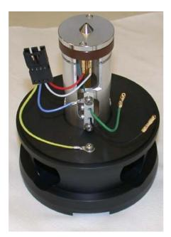
Figure 60 Ion optics assembly
