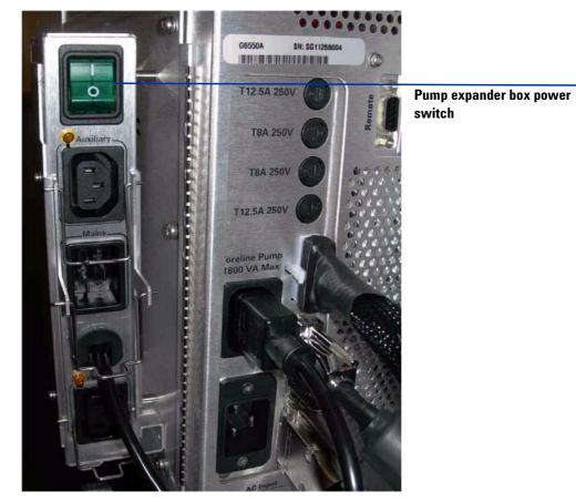
**Figure 6** 6550 power connections and pump expander box behind service panel
