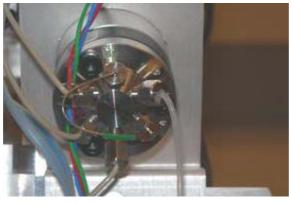
Figure 1 Divert valve with port position indicators
