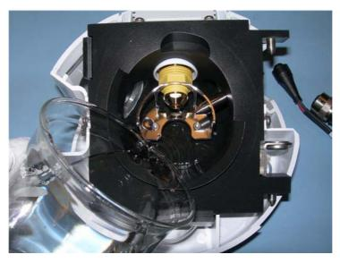
Figure 22 Filling the spray chamber
