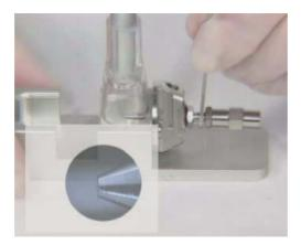
Figure 41 Adjusting the needle holder
