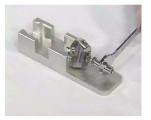
**Figure 36** Installing the nebulizer in the adjustment fixture
