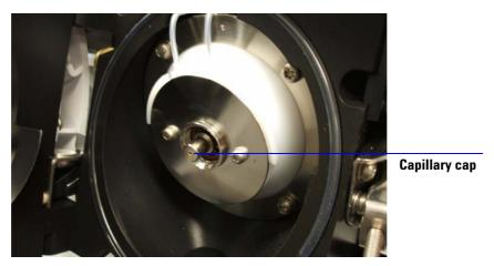
Figure 23 End of capillary cap
