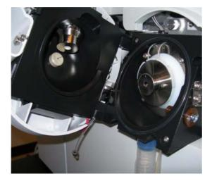
Figure 34 Opened spray chamber
