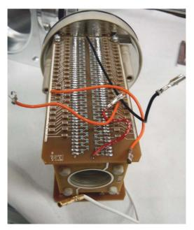
**Figure 72** High pressure ion funnel on top of a clean cloth.
