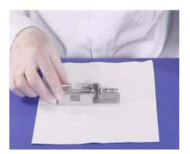
Figure 26 Electrospray nebulizer needle in needle holder
