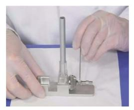
Figure 40 Installing the nebulizer in the adjustment fixture
