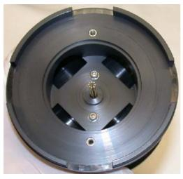
Figure 62 Octopole rods extending through Skimmer Spacer.
