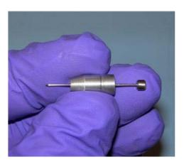
Figure 46 Replace the APCI corona needle.
