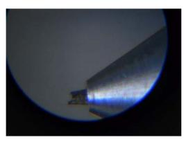
Figure 12 Corroded needle in nebulizer
