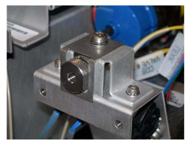
**Figure 4** Inlet filter assembly
