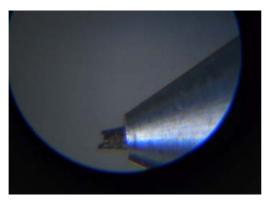
Figure 27 Corroded needle in nebulizer
