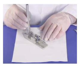
Figure 32 Nebulizer installation with adjustment fixture
