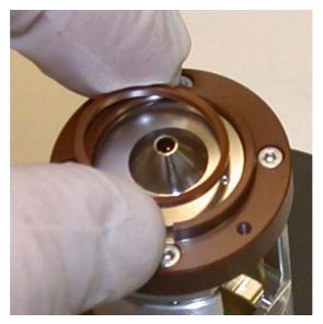
Figure 66 Spacer insulator
