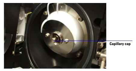
Figure 8 End of capillary cap
