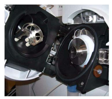
Figure 6 Opened electrospray spray chamber
