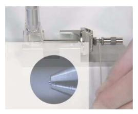
Figure 16 Adjusting the needle holder
