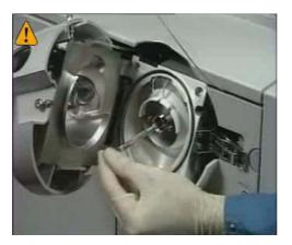
Figure 56 Reinstalling the capillary
