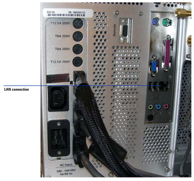
**Figure 5** 6520/6530/6538/6540 gas, LAN, and power connections behind service panel
