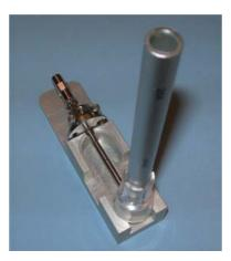
Figure 11Electrospray nebulizer needle in needle holder
