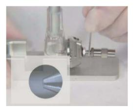
Figure 33 Adjusting the needle holder
