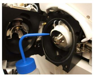
Figure 9 Rinsing the area around the spray shield
