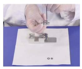
**Figure 49** Tightening the union screw to compress the ferrule
