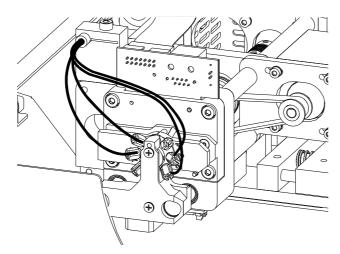
Figure 53 Routing capillaries
