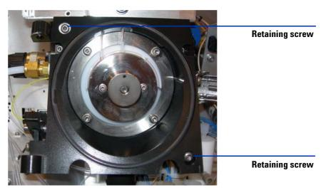
Figure 17 Remove the retaining screws. (6510 and 6520)
